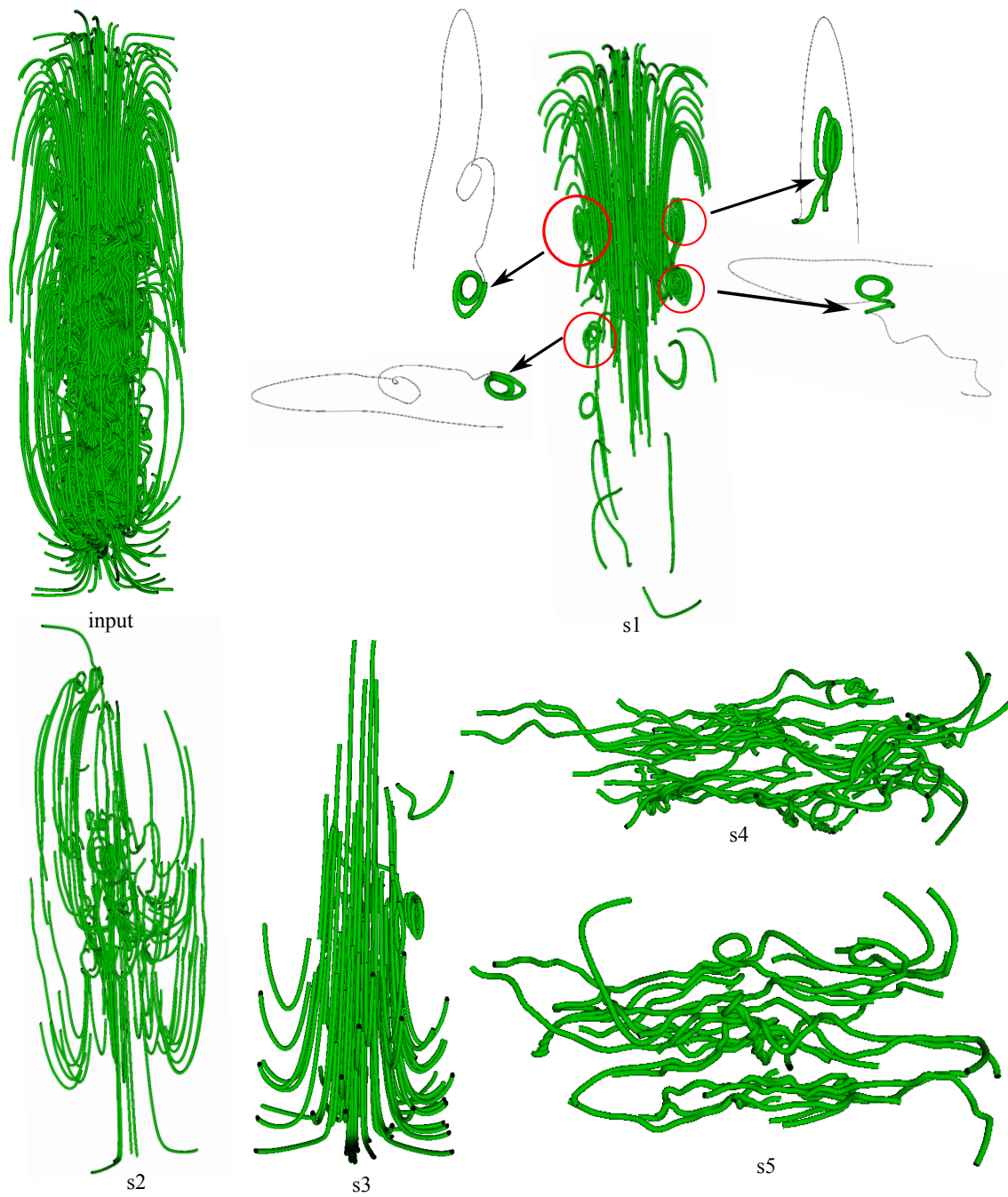
Figure 4.12: Five ( s_1 - s_5 ) clusters of streamline segments of the solar plume data set are shown. Notice how the interesting features such as spirals and turbulent features are successfully extracted.
