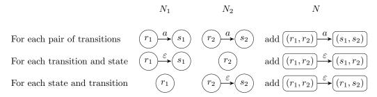
The first case is similar to the DFA intersection construction: Both  $N_1$  and  $N_2$  read an *a* symbol. But the handling of  $\varepsilon$ -transitions is new: In the second case,  $N_1$  follows an  $\varepsilon$ -transition while  $N_2$  does nothing; in the third case,  $N_2$  follows an  $\varepsilon$ -transition while  $N_1$  does nothing.
