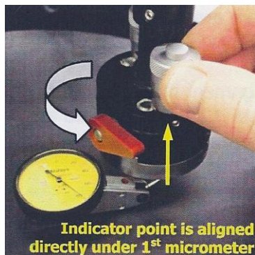
Figure 12: Indicator point aligned with the 1 st micrometer.
