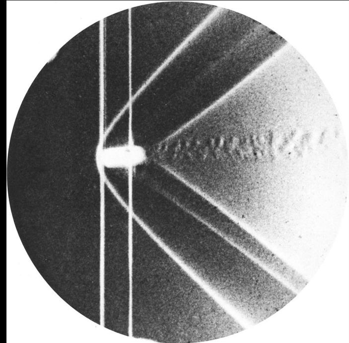
1886-1887, Study of Shock Waves Using Schlieren Photography
