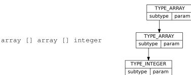
To express the type of a function, we use subtype to express the return type of the function, and then connect a linked list of param\_list nodes to describe the name and type of each parameter to the function.
