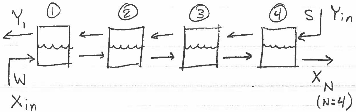
We are stripping a dilute solute from a water stream  $W$  by contacting
