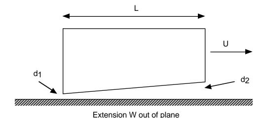
2. For a sliding block of dimensions  $L=10 \mathrm{cm}$ ,  $W=30 \mathrm{cm}$ , and  $d_2$ - $d_1=0.1 \mathrm{cm}$  (e.g., a fixed inclination angle), determine the velocity U at which the block can support a weight of  $100 \mathrm{kg}$  while maintaining a minimum separation  $d_1=0.01 \mathrm{cm}$ . Take the fluid viscosity to be 0.5 poise.
