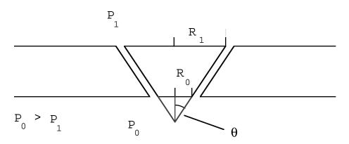
Hint: Assuming parrallel flow in the gap, use Bernoulli's equation and continuity to determine the velocity in the gap.
