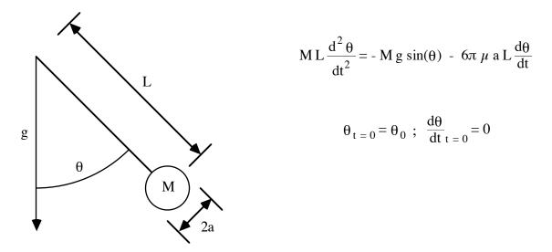
a. By choosing an appropriate reference time scale, render the equation and initial condition dimensionless. Show that the dimensionless solution depends on only two dimensionless groups. What are the physical meanings of these parameters?
