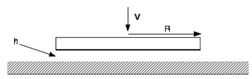
4. By taking the divergence of the equations of motion and applying the equation of continuity, prove that  $\nabla^2 p = 0$  for an incompressible fluid undergoing flow at zero Reynolds number. Use index notation only, and note that the  $\nabla$  and  $\nabla^2$  operators commute.
