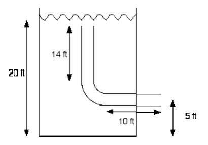
3. A recycle pump is installed on a CSTR as depicted below. Where should the pump be placed on the recycle stream? If we want to throttle the flow from the pump, where should the metering valve be placed? Briefly justify your answer.
