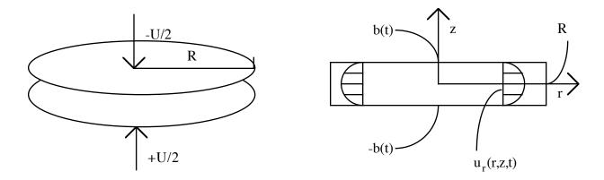
The two disks of radius R are approaching each other with velocity U (e.g., the upper disk moves with velocity -U/2 and the lower with velocity +U/2 in the z direction). As the disks approach each other, the fluid between the disks will be squeezed out.
