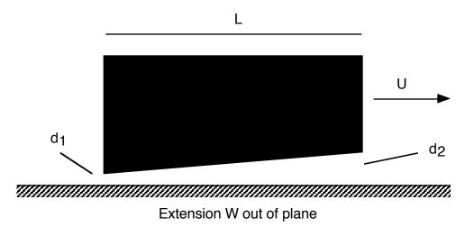
2. For a sliding block of dimensions L = 10cm, W = 30cm, and  $d_2$ - $d_1 = 0.1$ cm (e.g., a fixed inclination angle), determine the velocity U at which the block can support a weight of 100kg while maintaining a minimum separation  $d_1 = 0.01$ cm. Take the fluid viscosity to be 0.5 poise.
