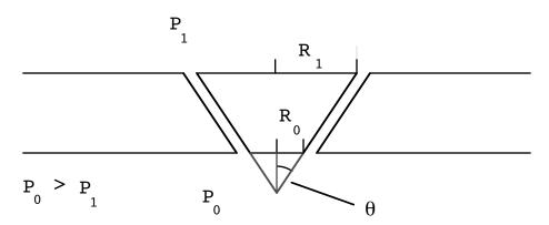
Hint: Assuming parallel flow in the gap, use Bernoulli's equation and continuity to determine the velocity in the gap.
