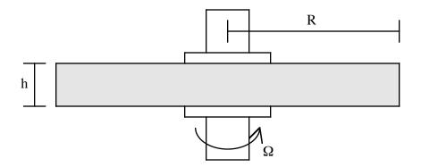
3. A common problem in determining the rheological behavior of suspensions of particles in viscous fluids is measuring the viscosity of the suspensions in a parallel plate viscometer. This presents difficulties, however, if the particle density is somewhat greater than the fluid density since the particles would tend to settle, affecting the observed viscosity. As a budding rheologist, you are asked to estimate the magnitude of this effect. So:
