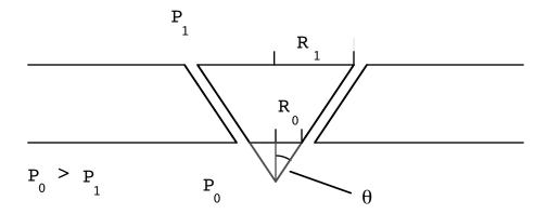
Hint: Assuming parallel flow in the gap, use Bernoulli's equation and continuity to determine the velocity in the gap.
