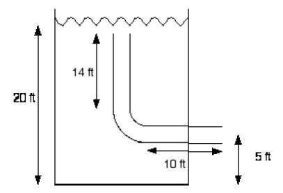
3. A recycle pump is installed on a CSTR as depicted below. Where should the pump be placed on the recycle stream? If we want to throttle the flow from the pump, where should the metering valve be placed? Briefly justify your answer.
