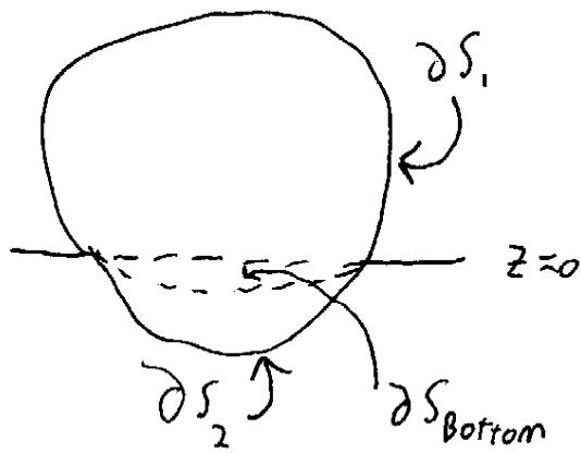
If we add and subtract the force = (pressure) · (area) integral over  $\partial S_{\text{Bottom}}$ , we can create a new closed integral surface.
