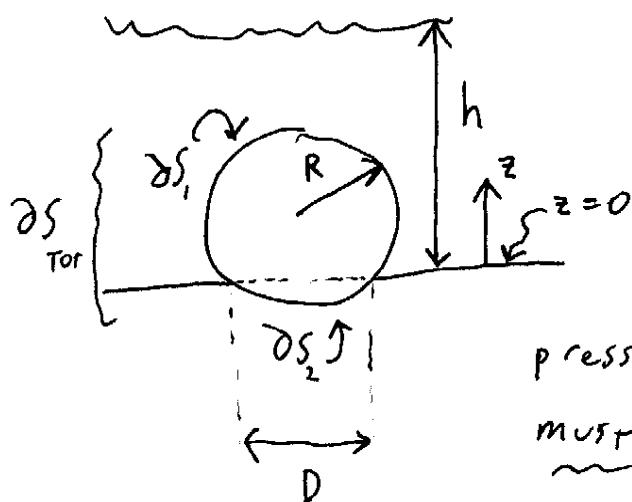
We know that the pressure exerted by the fluid acts normal to the surface of ball. If we sum up the forces associated with that pressure over the entire surface, they must sum to zero for the ball to remain stationary.
