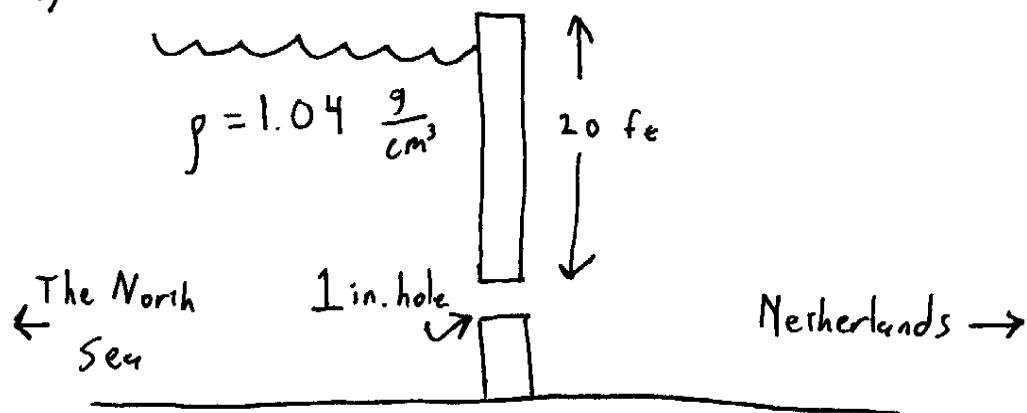
a.) Find the force necessary to plug a 1 inch hole.
