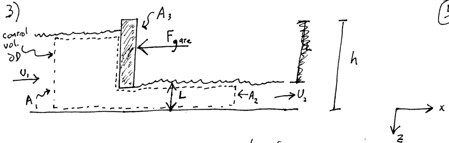
• Derive an expression for the force per unit width to keep the gate in place.
