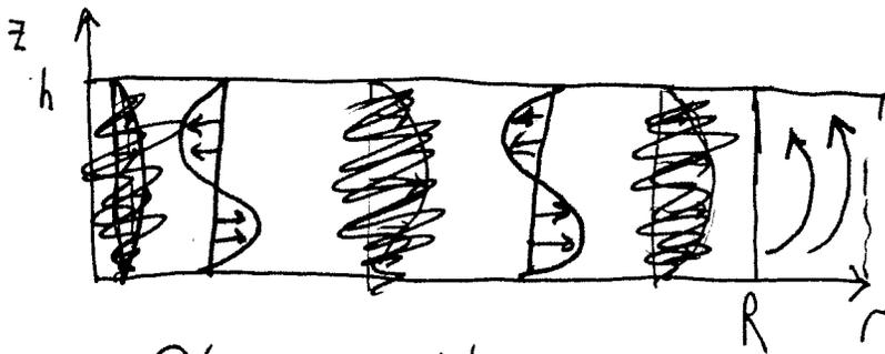
Backflow is the result of continuity. Fluid is thrown outward at rotating plate, and returns inward near the stationary plate. There is a strong turning current at the outer edge - and if surface tension isn't strong enough to confine it, the lab gets sprayed!
