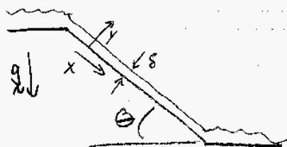
If the fluid is viscous, it will rapidly reach some constant thickness  $\delta$ , and some steady velocity profile. What is the relationship between  $Q/W$ ,  $u$ ,  $\delta$ ,  $\theta$ ,  $\mu$ ,  $g$ , and  $\rho$ ?? Just apply the Navier-Stokes equations!
