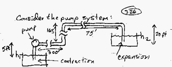
Suppose we have all 4" ID smooth pipe, and we want a flow rate  $Q = 42 \text{ ft}^3/\text{min}$ . What is the required power of the pump?
