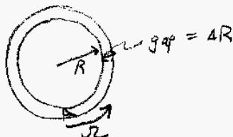
By rotating the outer cylinder you deform the fluid in the gap and exert a torque on the inner cylinder. This torque is used to calculate the viscosity!
