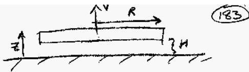
The flow in the narrow gap  $H/R \ll 1$  will resist the upward motion of the disk. We want to calculate this force. The flow is three-dimensional, but  $u_\theta = 0$  & we can neglect  $\theta$  derivatives! Let's start with the C.E.:
