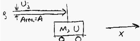
A jet of water of diameter  $D$  & velocity  $U_j$  impinges on the plate. What is the force on the plate as a function of  $U$ ? What is the velocity of the car as a function of time?
