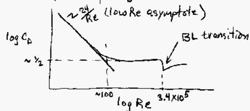
The abrupt transition at  $Re \approx 3.4 \times 10^5$  results from the transition of the BL to turbulence, delaying separation, giving an increase in pressure recovery and reducing drag  $\sim 6$  fold! On a baseball this transition is triggered at a lower  $Re$
