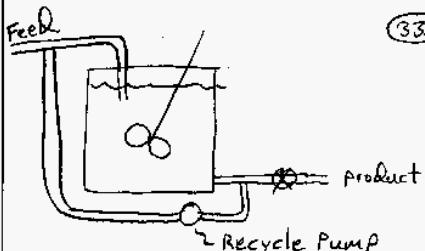
Suppose we want to size the pump for the recycle stream. We can represent the head losses & flow rates as an electrical network!
