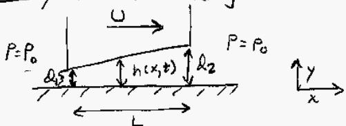
If  $H \gg d_1, d_2, L$  we can use lubrication theory to calculate the upward force on the block for some  $U, d_1, d_2, L$ , etc.
