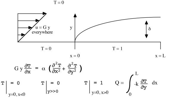
2. Boundary layer growth with suction: One technique used to control the rate of boundary layer growth on airplane wings is suction -- the wing (or plate) is porous, and fluid is sucked out of tiny holes which has the effect of keeping the boundary layer attached and preventing separation. In this problem we will examine the simple case of
