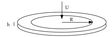
In this case the fluid of volume V is inserted between the plates, and the upper plate falls with a velocity U in the -z direction. The lower plate is fixed, so the gap width h is governed by the simple equation:
