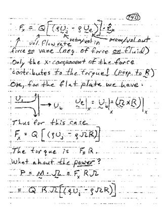
Note that the torque is maxed when  $S^2 = 0$  but the power is zero!
