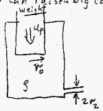
For a given motion of the piston what is the flow rate thru the sutlet pipe? For a given weight of car, what is the pressure in the pipe?
