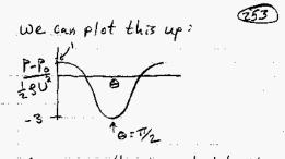
We can use this to calculate the Drag (f.ex) on the cylinder!
