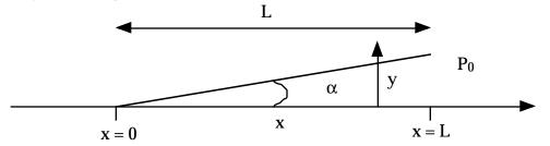
a. Set up the equations and boundary conditions governing this problem (Hint: Use a length scale  $H = \alpha L$  and velocity scale  $V_c = L (d\alpha/dt)$  in the y direction, and recall that from trigonometry tan  $\alpha \approx \sin \alpha \approx \alpha$  for  $\alpha << 1$ . Remember that the fluid displaced by the closing wedge has to squish out in the x direction).
