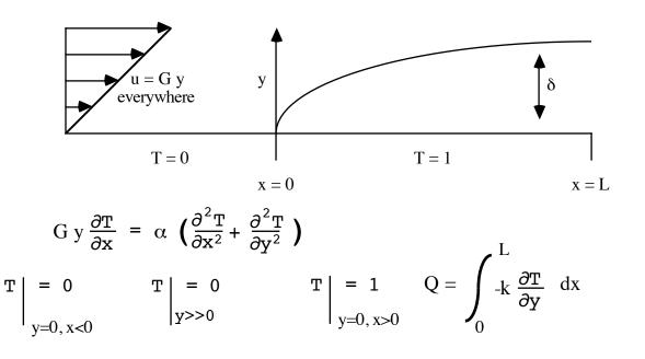
2. Boundary layer growth with suction: One technique used to control the rate of boundary layer growth on airplane wings is suction -- the wing (or plate) is porous, and fluid is sucked out of tiny holes which has the effect of keeping the boundary layer attached and preventing separation. In this problem we will examine the simple case of uniform flow past a flat plate where the vertical suction velocity is given by the power-law relation:
