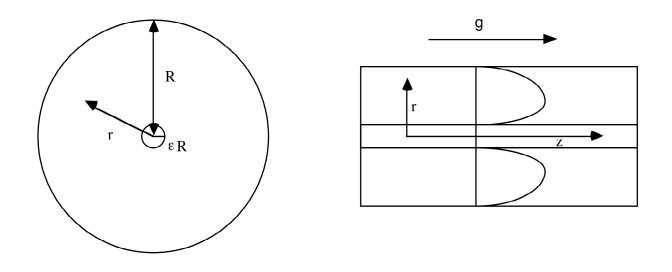
3. Core-Annular flow is an important technique for reducing the pressure drop for pumping a viscous fluid such as a heavy oil. The idea is that the viscous oil is surrounded by a narrow sheath of fluid with much lower viscosity (such as water). Because most of the shear would occur in this narrow region next to the wall, the stress and pressure drop is much lower for a given flow rate. Here we solve this problem.
