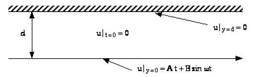
we wish to examine the influence of fluid inertia on the stress measured at the lower plate.
