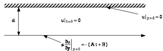
In this problem we are measuring the viscosity by looking at the effect of a linear ramp in the shear stress. The entire system is initially at rest, and at time t = 0 a shear stress given by  $\tau$  = - (A t + B) is applied to the lower wall. The velocity U of the lower wall is measured as a function of time, with the apparent viscosity being defined as  $\mu_{app} = \tau d / U$  where d is the gap w idth.
