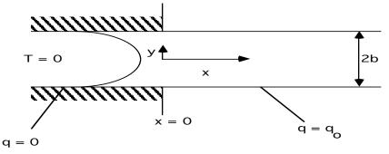
a. (10 points) Render the problem and boundary conditions dimensionless. Show, by rendering x dimensionless such that x-convection balances y conduction, that for sufficiently high velocities conduction in the x-direction is negligible.
