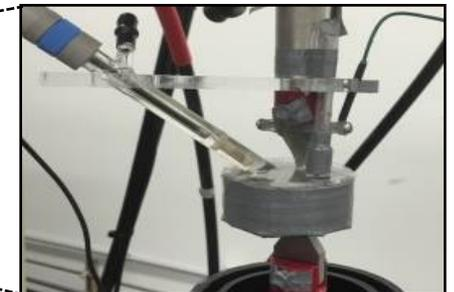
Electrochemical corrosion cell made of plexiglass
