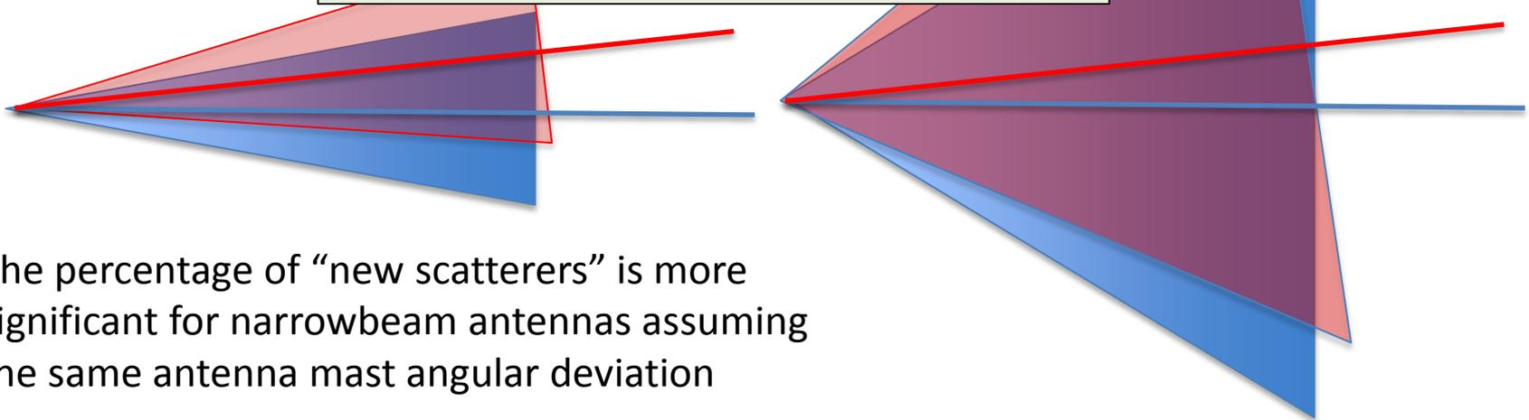
The percentage of “new scatterers” is more significant for narrowbeam antennas assuming the same antenna mast angular deviation
