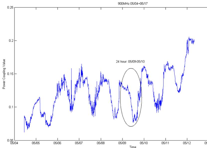
The daily cycles are induced by temperature and subsurface water level. The high-frequency noise is likely the result of wind and/or human activity
