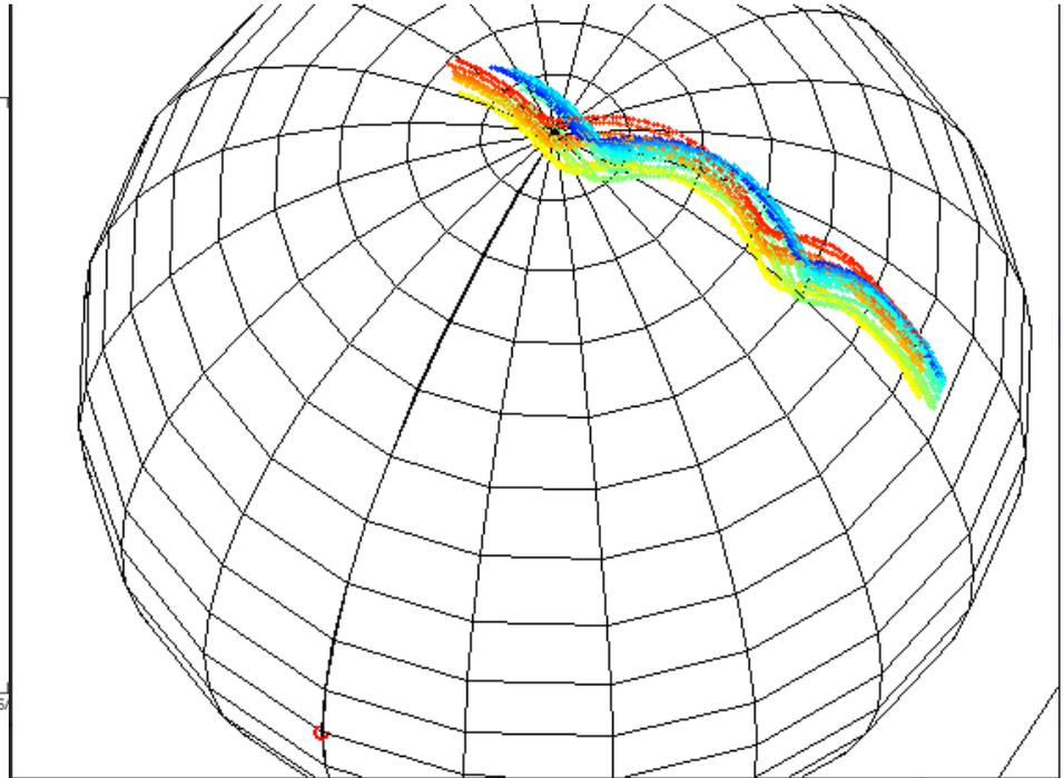
Color-coded time response shows how the PMD curves vary over the day-long cycle period. The curves have been averaged.
