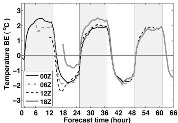
FIG. 19. Bias error of simulated 2-m temperature from the 1.11-km domain with various initialization times. The forecasting period for all forecasts is 48 h.
