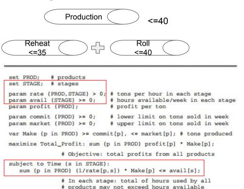
Figure 1-6a: Additional resource constraints (steel4.mod).
