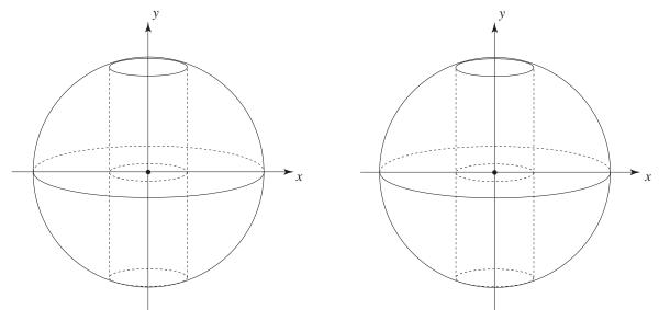
1. With the "shell" method, by revolving a vertical area element around the y-axis. Start by drawing a vertical area element (into the sphere on the left) and determine its upper and lower limits. Let dx be its (thin) width. Then find and expression for the volume of revolution that this element generates. Put the definite integral into the box.
