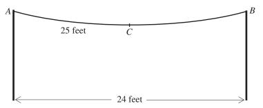
1. A laundry bag containing 35 pounds of wet laundry is attached to the clothesline at its midpoint C. Compared to the weight of the laundry, the weight of both the clothesline and the laundry bag are negligible.
