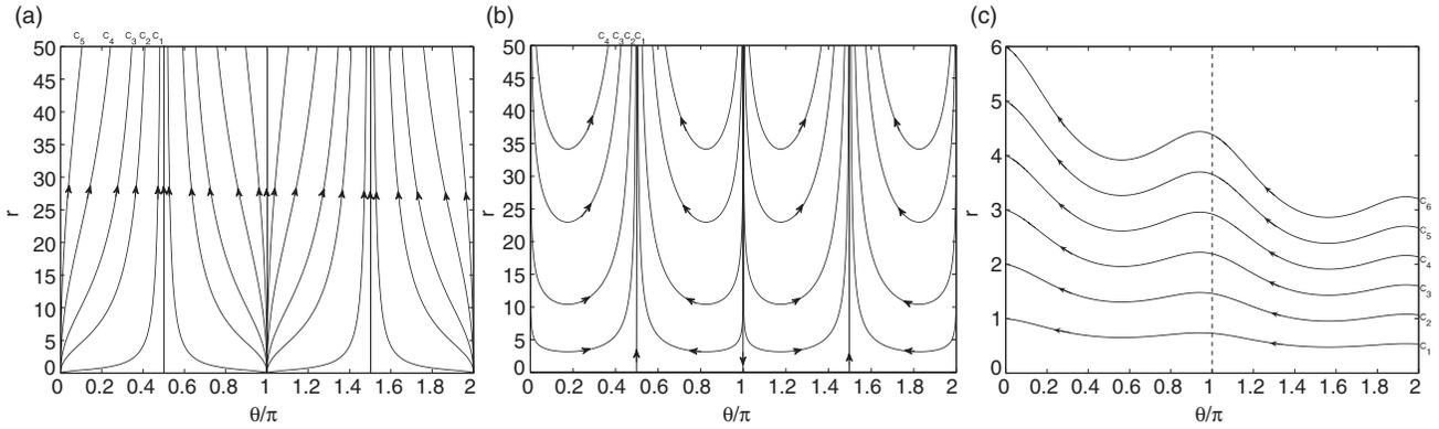
Figure 1. The phase diagrams of second-order LTI systems in polar coordinates: (a) node, (b) saddle point and (c) focus.
