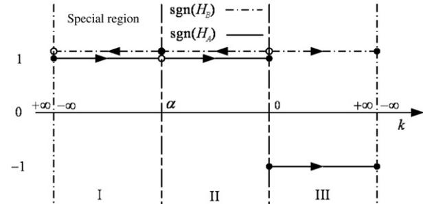
Figure A1.  $S_{12}$ :  $N(k)$  does not have two distinct real roots, the switched system is unstabilisable.
