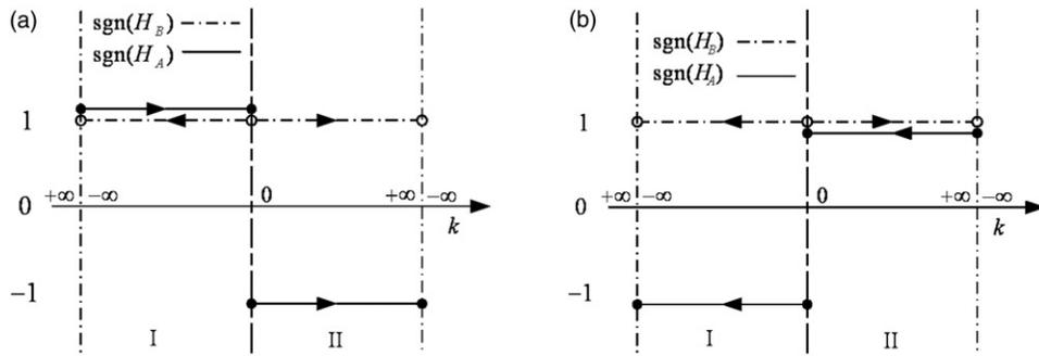
Figure A4.  $S_{13}$ :  $N(k)$  does not have two distinct real roots, the switched system is unswitchable: (a)  $\det(P_3) < 0$  and (b)  $\det(P_3) > 0$ .
