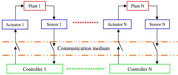
Fig. 1. Communication of controller-plants through a shared communication medium.
