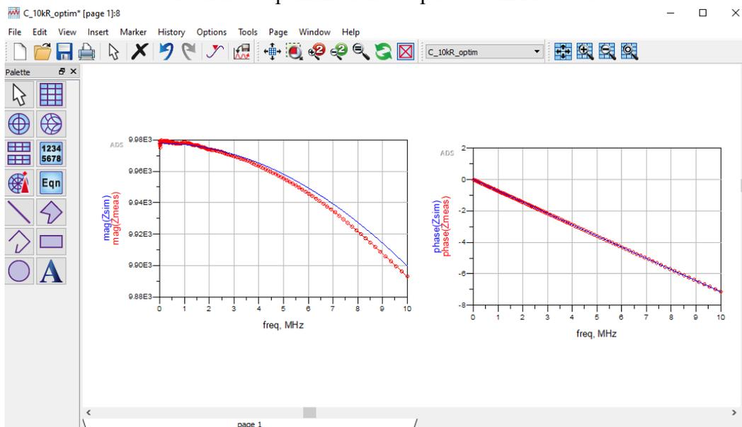
Screenshot: Comparison of measurement (red) and model (blue) for 10 kΩ resistor. Note: the y-axis scale covers a very small range of values.
