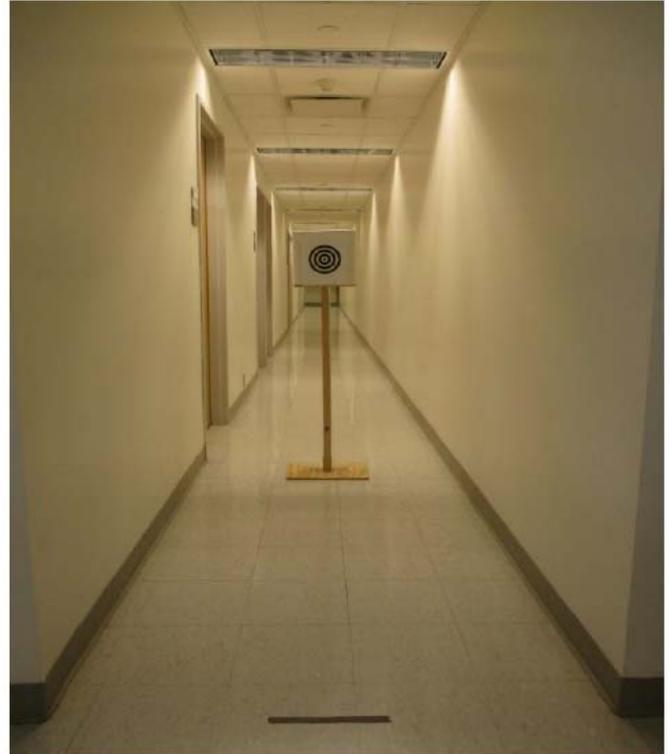
**Figure 3.** Experiment 2 set-up. Target was placed at five points along a hallway. Participants stood at center line and reported the distances under either the laser or baton conditions.
