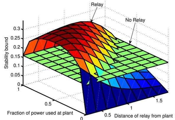
Fig. 3. Sufficient condition bound as a function of fraction of power used at the plant and distance of relay from plant.
