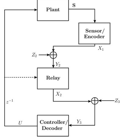
Fig. 2. Block diagram for an unstable plant being controlled by a controller across an AWGN cascade channel
