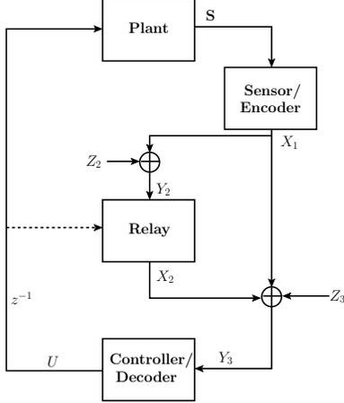
Fig. 1. Block diagram for an unstable plant being controlled by a controller across an AWGN relay channel
