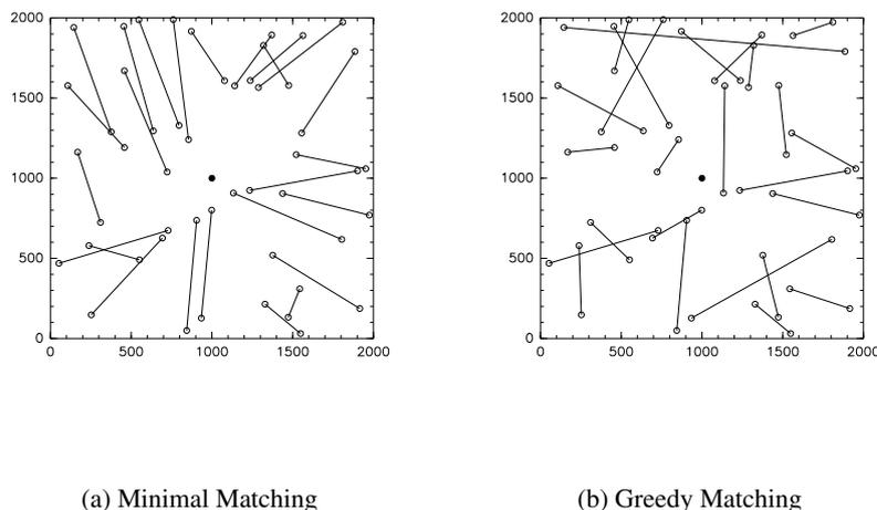
Figure 1.4. Matching algorithm results for an example network: (a) minimal matching, (b) greedy matching. Terminals are indicated by circles, and matched terminals are connected with lines.
