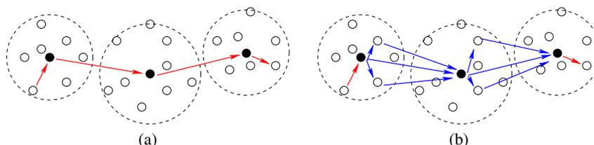
Figure 1.5. Clustering with (a) direct transmission and (b) cooperative diversity transmission.
