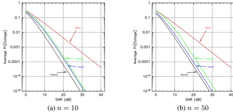
Figure 1.3. Matching algorithm performance in terms of average outage probability vs. received SNR (normalized for direct transmission).
