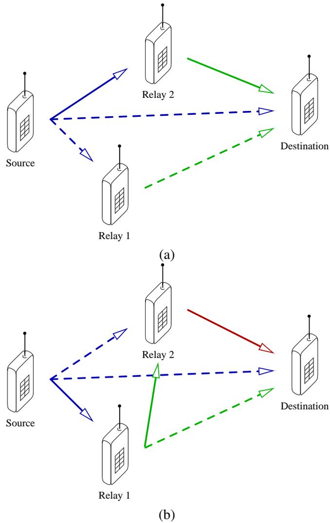
Figure 1.1. Illustration of cooperative wireless transmission with (a) parallel relays and (b) serial relays. Colors indicate transmissions that occur in different time slots or frequency bands. Solid arrows indicate transmissions that are utilized in traditional multihop transmission. Cooperative communications utilizes transmissions corresponding to both solid and dashed arrows by having the appropriate receivers perform some form of combining of their respective incoming signals.
