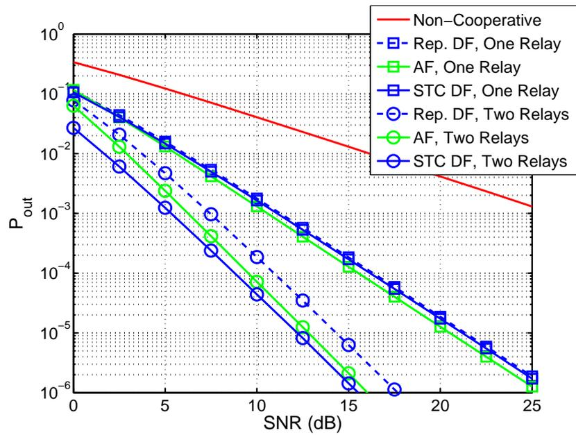
Figure 1.2. Example outage performance of non-cooperative and cooperative transmission computed via Monte Carlo simulations. The model has: path-loss with exponent  $\alpha = 3$ , independent Rayleigh fading, network geometry with relays located at the midpoint between the source and destination, spectral efficiency  $R = 1/2$ , and uniform power allocation.
