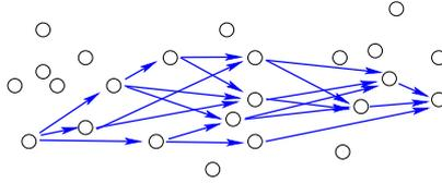
*Figure 1.6.* Illustration of multi-stage cooperative transmission. Downstream receivers can combine signals from all upstream transmitters. Only one complicated “link” is presented to the network layer.
