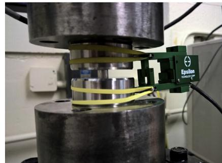
**Fig. 2.** Experimental setup for uniaxial compression experiments.
