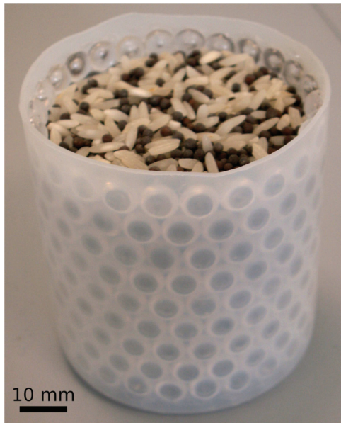
FIG. 1. (Color online) Scanning container filled with 50% weight of spheres to ellipsoids. The hemispherical beads (3 mm radius) on the boundary of the container are used to minimize boundary effects. The container is 65 mm in height and 62 mm in diameter.
