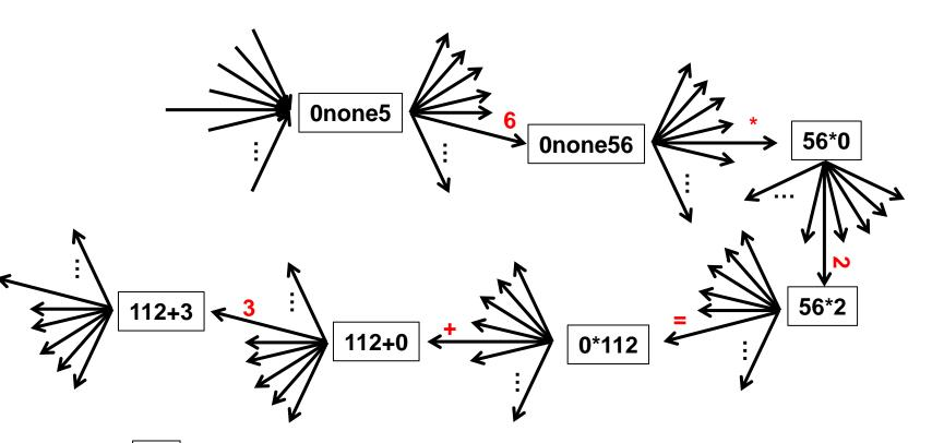
is "state" where "i" is saved #, j is displayed #, and "x" is last operator "none" represent no operation pushed since power on
