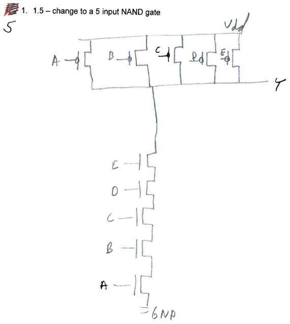
2. 1.6 – this should be a transistor diagram of a single gate, not a combination of simpler NAND/NOR gates.
