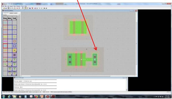
• Repeat for pMOS but place contacts between the polys also. Note: you may want to build the center row of contacts "outside" first, then wire and position. You may also want to expand the space between the two p-types to stop errors.
