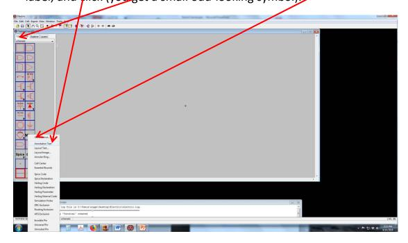
• Double click on the symbol, type in a name of the cell ("NAND2"),, and when done move the cursor away and click to exit the text editing. This leaves NAD2 with an "X" thru it. Either Ctrl-I or Edit/Properties/Object Properties, and then set Text Size to 20, and units to "Points". Apply and hit OK.
