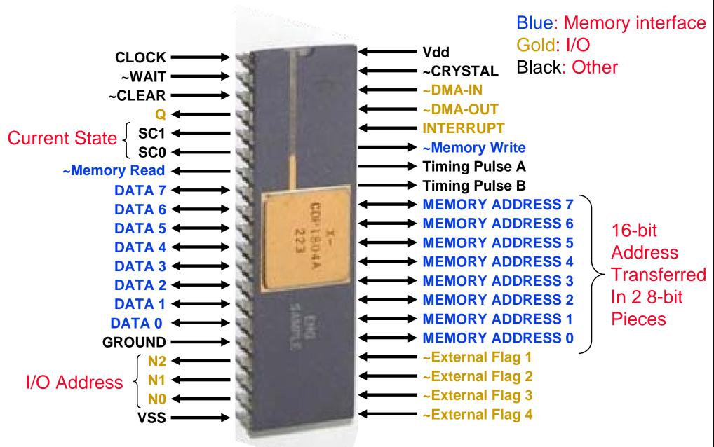
Note: a "~" in front of a signal means that it is "active low" i.i. a "0" indicates the signal is "active"
