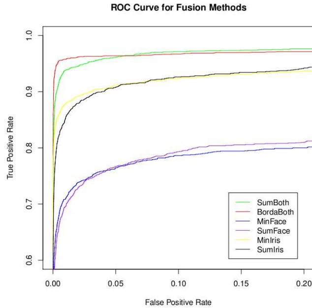
**Fig. 9** ROC curves for the various fusion methods using the optimal tested parameters for each. The BordaBoth method shown is the BordaBoth-Exponential method.
