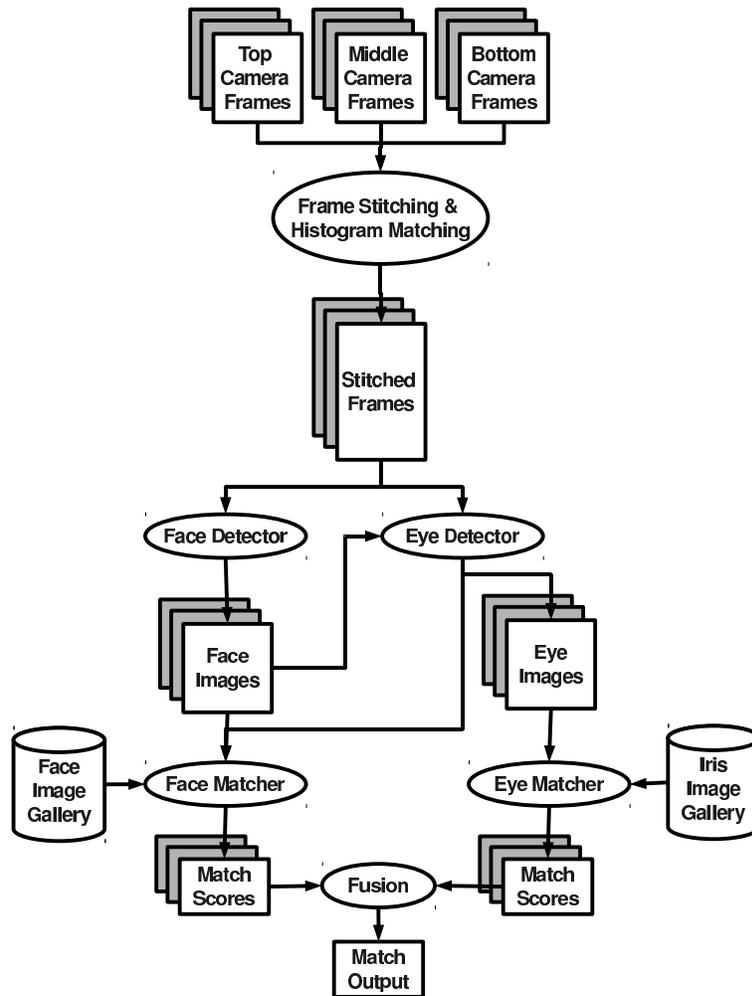
**Fig. 3** A diagram of the pipeline used in the proposed multi-biometric system.
