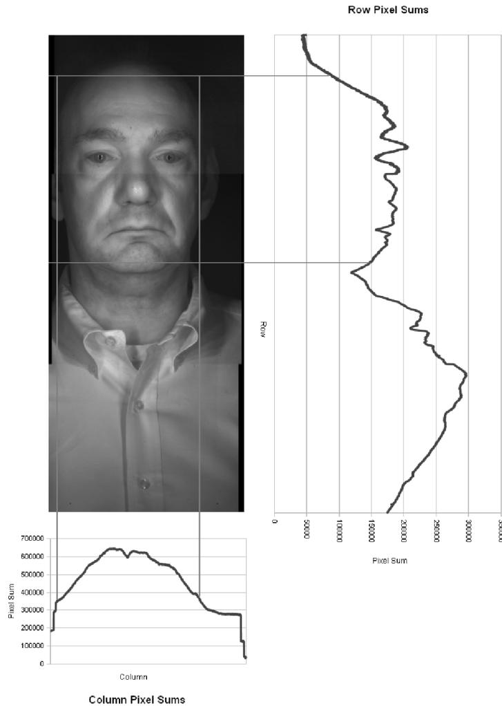
**Fig. 5** Example of the image projection technique used to estimate the location of the face during eye detection. The graphs on the right and bottom of the image represent the summations of the pixel values in each row or column, respectively. The projected lines represent the face boundaries determined using appropriate thresholds.
