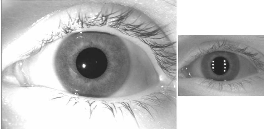
**Fig. 6** Images of the same iris image using the LG4000 (left) and the IOM (right). The IOM image shown on the right represents a well-focused IOM iris image.
