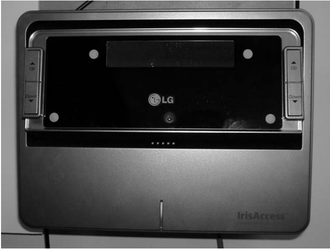
Fig. 5. Images in our data set were captured using this LG4000 iris camera [13].
