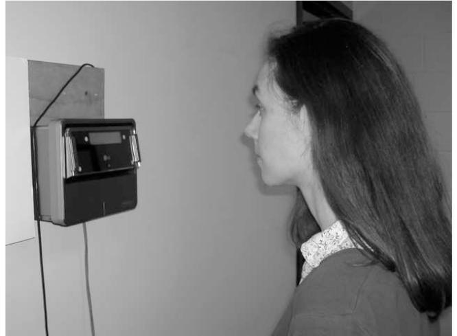
Fig. 7. The LG4000 iris camera captures images of both eyes at the same time.
