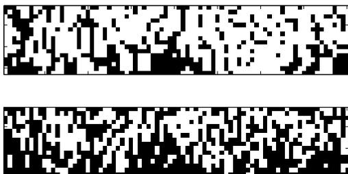
Fig. 2. The consistency of each bit in the iris code is dependent upon a combination of the iris texture at a certain position and the filter used to analyze that texture. These two fragile bit patterns both correspond to the same iris, but a different filter has been used, and consequently, different fragile bit patterns emerge. Black regions represent fragile bits in the iris code, and white regions represent consistent bits.
